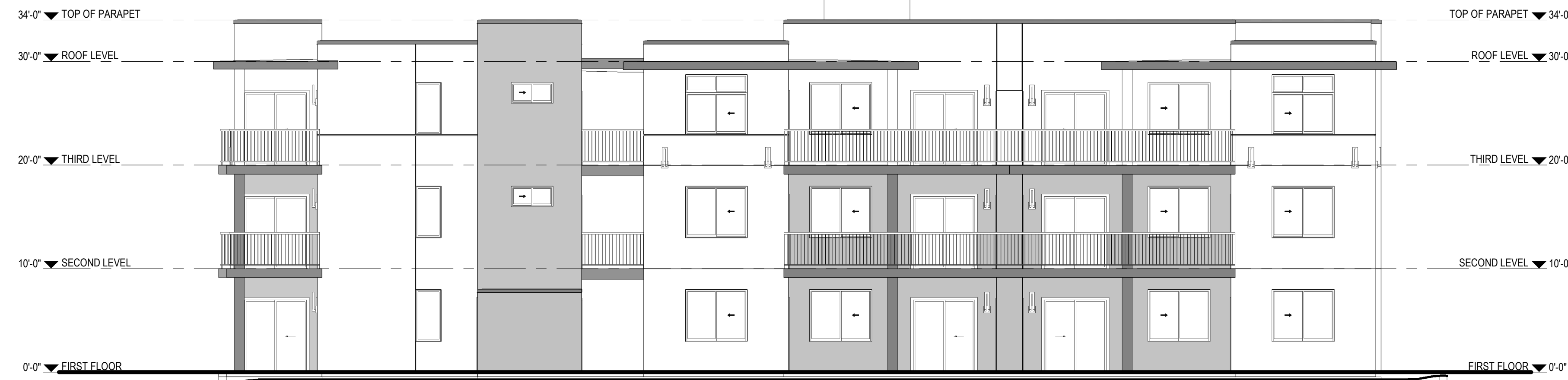
1 APARTMENT BLDG NORTH ELEVATION Ref: A-101 / Scale: 1/8" = 1'-0"
